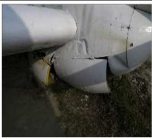
The damaged propeller blades and lower left engine cowling
