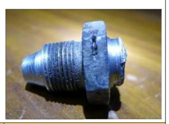
Picture of the failed hydraulic fitting
