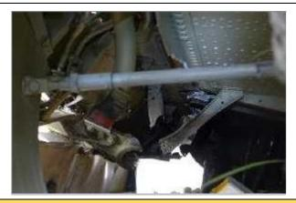
Collapsed & buckled left MLG and Broken / Wrecked MLG under wing frame
